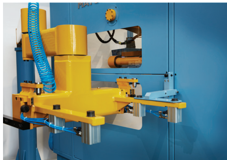
DISA Quick Matchplate Changer (QMC) with safety locking on DISA MATCH 20/24
