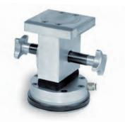
This accessory is used for gassing the test samples in the core box.
