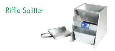
When used in conjunction with the Microsplitter (Model 42106B), this accessory is used to prepare a representative sample of unbonded foundry sands for sieve analysis testing. Fourteen (14) 1/2" chutes divide the sand accurately in half to provide representative sand samples down to 125 grams.
