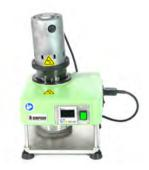
The Rapid Sand Washer is used to ensure correct and repeatable test results when preparing sand samples for the AFS Clay Tester (Model 42131). This sand washer uses highspeed agitation to remove all clay from the sand grains within the molding sand sample.
