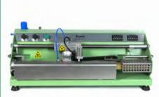
This tester measures the temperature at which shell resin coated sands melt and adhere to a heated bar. The melting temperature of the sand is considered the melt point or stick point.
