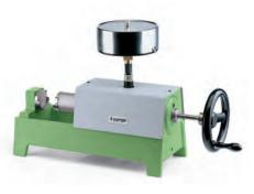
This hand-driven strength machine is used to determine the strength properties of clay and/or chemically bonded foundry sand specimens. The device has the capability to run five different sand strength tests with additional fixtures and accessories that are easy to connect to the instrument.
