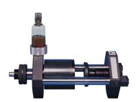
This accessory is a force multiplier that, when used with the Electronic Universal Sand Strength Machine (Model 42104), can perform a compression strength test on a standard AFS  $2" \times 2"$  (50mm x 50mm) sand specimen with a compression strength range of 250-3100 PSI (170-210 N/cm2).
