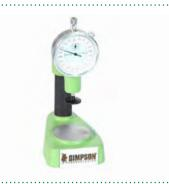
This accessory measures the deformation of a clay bonded sand specimen after a compression strength test is done on the Electronic Universal Sand Strength Machine (Model 42104). Deformation is the change in the length of the sand specimen before and after the compression test.
