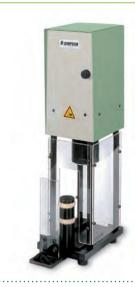
This instrument gently ejects the sand specimen from the specimen tube ensuring high repeatability.
