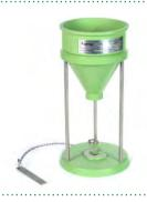
This accessory assists in filling the specimen tube for compactability tests. It assures that properly riddled sand fills the specimen tube from a standard and fixed distance. Both the Digital Pneumatic Sand Squeezer (Model 42160) and the Sand Rammer (Model 42100) use this accessory.
