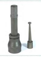
When using this device as an accessory to the Digital Absolute Permmeter (Model 42105), the base permeability of loose porous sand masses can be determined.
