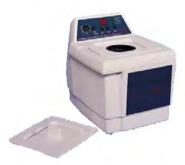
This cleaner is used with the Methylene Blue Clay Tester (Model 42108) to scrub a sand sample before the addition of methylene blue dye.
