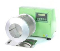
The friability of clay bonded foundry molding sand can be determined by using this instrument to measure the ability of compacted molding sand to resist abrasion or scuffing within the first few millimeters at the surface of a prepared mold.
