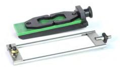
This accessory is used to determine the tensile strength of shell/croning coated mold and core sands when mounted on the Electronic Universal Sand Strength Machine (Model 42104).
