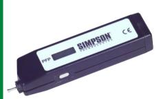
This portable electronic handheld tester is used to determine the mold strength on a finished mold.
