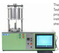
The High Temperature Compression Tester is used to determine the hot strength properties of a molding sand sample. The instrument measures both hot compressive strength and hot deformation.
