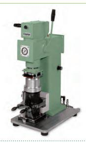
The Labjet is designed to manufacture standard transverse test specimens. When using the corresponding attachments, test specimens can be made using gas- and heat-cured core and molding sand.
