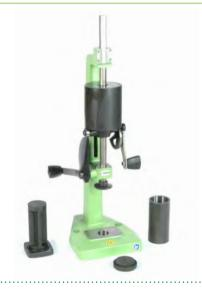
The Sand Rammer is used to prepare standard AFS 2" x 2" (50mm x 50mm) cylindrical sand specimens. It is also used to determine the compactability of prepared clay bonded molding sand used in a foundry.
