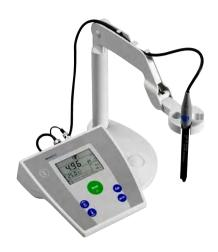
The Acid Demand Value (ADV) Tester measures the amount of basic material present in the sand that is soluble in a dilute acid solution.
