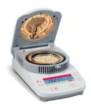
To determine the moisture content of green sand and other raw materials used within the foundry, this analyzer can be used.
