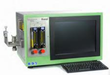
The Hot Distortion Tester is specifically designed to rapidly heat and measure any corresponding upward and/or downward deflections of a standard shell transverse sand specimen.
