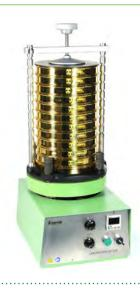
The sifter is used to determine the grain fineness and distribution of foundry sands.
