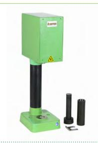
This instrument is used to prepare AFS standard sand specimens of clay bonded molding sand used for high temperature compression testing in the High Temperature Compression Tester (Model 42115).
