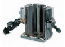
This accessory is used for manual or mechanical preparation of standard transverse test specimens.
