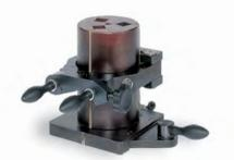
This accessory is used in the production of three transverse strength specimens using a gas-cured molding sand.
