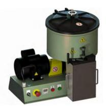
The Simpson Laboratory Muller is used to prepare mixtures of clay bonded foundry sands. The mulling conditions found in industrial mullers can be emulated on a smaller scale using this laboratory muller.
