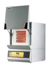
This furnace is used to measure the loss on ignition (LOI) and volatiles on both chemically and clay bonded foundry sands.
