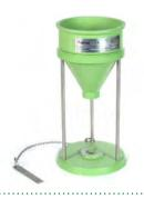
This accessory is required to fill the specimen tube for compactability tests. It assures that properly riddled sand fills the specimen tube from a standard and fixed distance.
