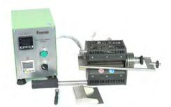
Measuring the hot tensile strength of shell/ croning sands can be performed using this accessory with the Electronic Universal Sand Strength Machine (Model 42104).
