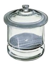
The desiccator is used to protect sand specimens from water vapor in the air during the cooling of samples after those samples have been heated in the Muffle Furnace (Model 42127).
