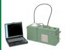
This instrument can be used to accurately measure the gas pressure generated over time from a foundry sand sample heated to a set temperature.
