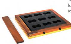
This core box makes standard specimens for tensile strength testing using self-curing (air-set) sands.
