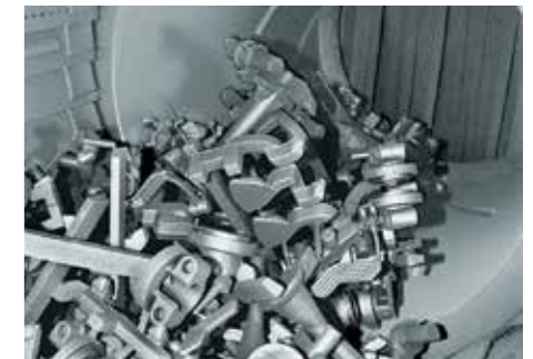
Parts in the outlet barrel after cleaning
