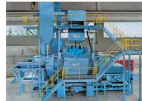
Blast cleaning machine with inlet and outlet vibratory conveyors
