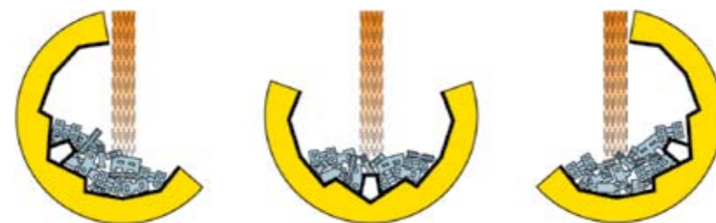
Rocking motion of the polygon-shaped trough about its longitudinal axis for gentle tumbling of the castings
