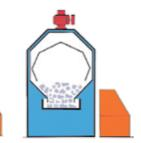
Unloading from the trough after it has turned into unloading position. The empty trough then continues to turn into loading position.
