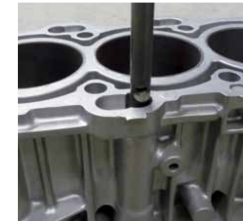
Inside blasting of crankcases
