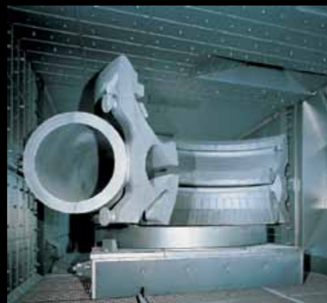
Blast cleaning (sand removal) of compressor housing
