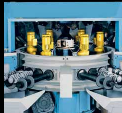
Fully automatic shot peening of more than 600 crank shafts / h on DS machine
