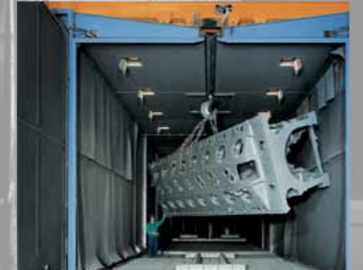
Blast house for a 80 tonne diesel engine block
