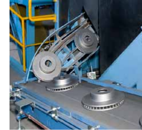
Process-safe blasting of single parts
