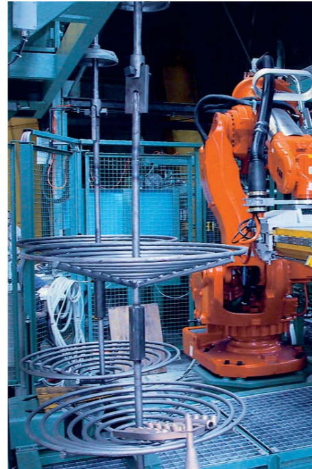
Robotic loading of hangers
