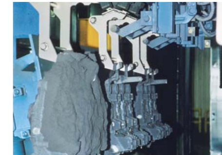
Hanger-type machine with monorail loop for desanding automotive components.
