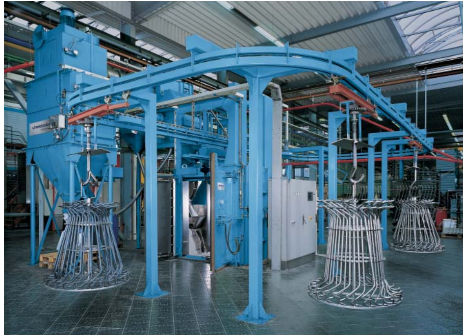
Hanger-type solution with monorail for shot peening of stabilizers for passenger cars
