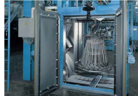
Hanger-type shotblast machine for through-feed operation
