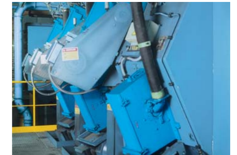
12 blast wheels, 37 kW each.
