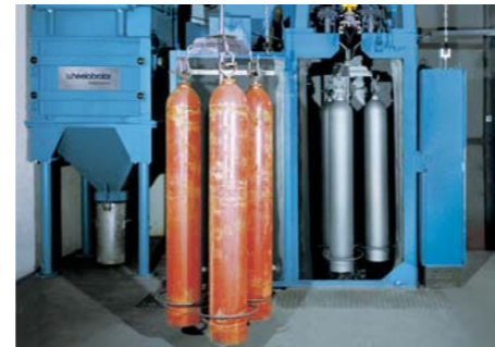
Hanger-type shotblast machine for reconditioning gas bottles
