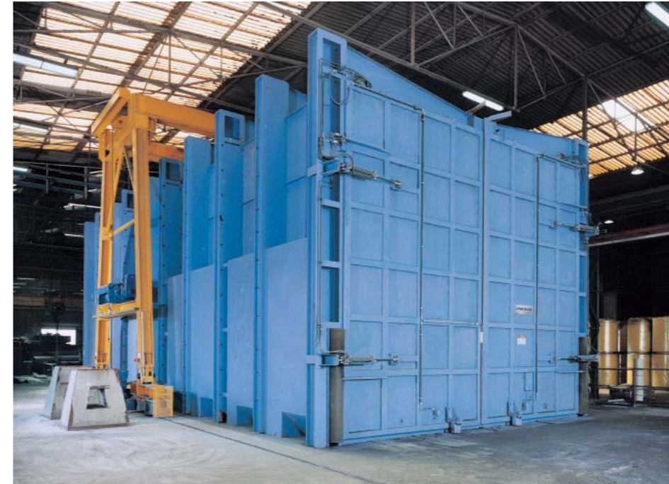
Blastroom with travelling crane for large and heavy parts.
