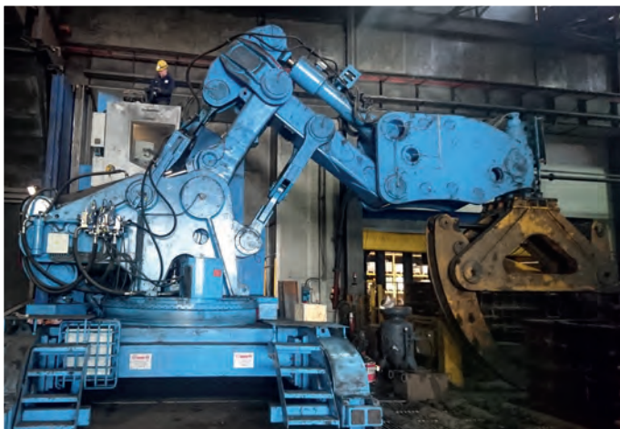
C20020 rail bound manipulator with 20 tonnes capacity.
