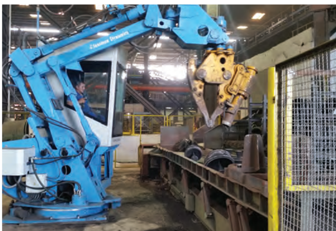
C620 manipulator with gripper mounted cannon.
