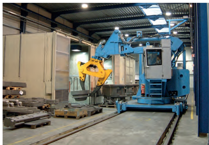
C5010 rail bound manipulator with 5 tons capacity
