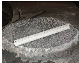
Flat surface at break-off point Konturunschädliche Bruchfläche
