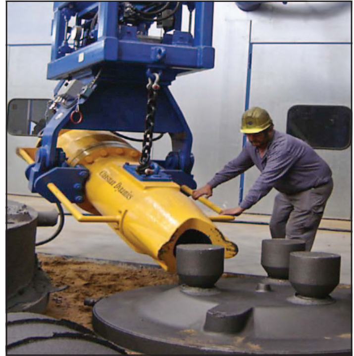
Drive/tilt hammer on to feeder. Positionieren hammer in Schussbereitschaft.
